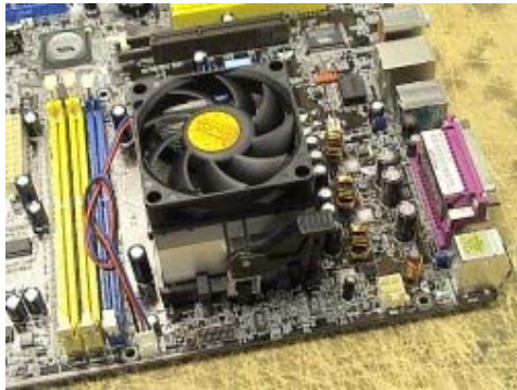
Installed HeatSink and Fan
